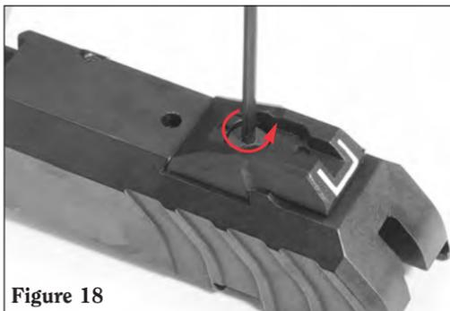
Lay the slide flat on a suitable working surface. With a 5/64" Allen wrench, remove the rear sight screw from the slide by turning it counter-clockwise (see Figure 18).
