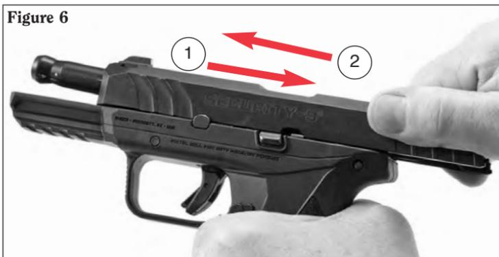
5. Retract the slide approximately 1/16" so the front of the slide aligns with the front of the grip frame. Pry loose the takedown pin using a non-marring armorer's tool or other flat, blunt tool (see Figure 7).
