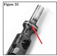
Make sure the extractor spring and extractor buffer spring are in place in the extractor (see Figure 36).
