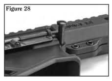
c. Lift the upper receiver off the lower receiver to do any additional cleaning.
