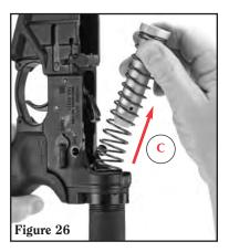
**WARNING:** Do not attempt to stretch or otherwise modify the buffer spring. Functional issues can result from modifications to the buffer spring.
