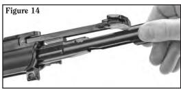
d. Grasp the rear of the bolt carrier assembly, remove it from the upper receiver, and set it aside.
