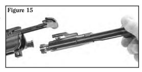
e. Grasp the charging handle and pull it rearwards until the handle stops, then slide the charging handle down (out of the cutout in the receiver) into the holt carrier
