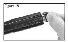
c. Remove the firing pin from the bolt carrier.
