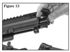
c. Pull the charging handle approximately halfway out of the upper receiver and stop. The bolt carrier assembly will follow the charging handle.
